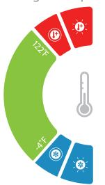
$Hot\ LED\ indicator Designed\ to\ indicate$ when internal battery approaches high
